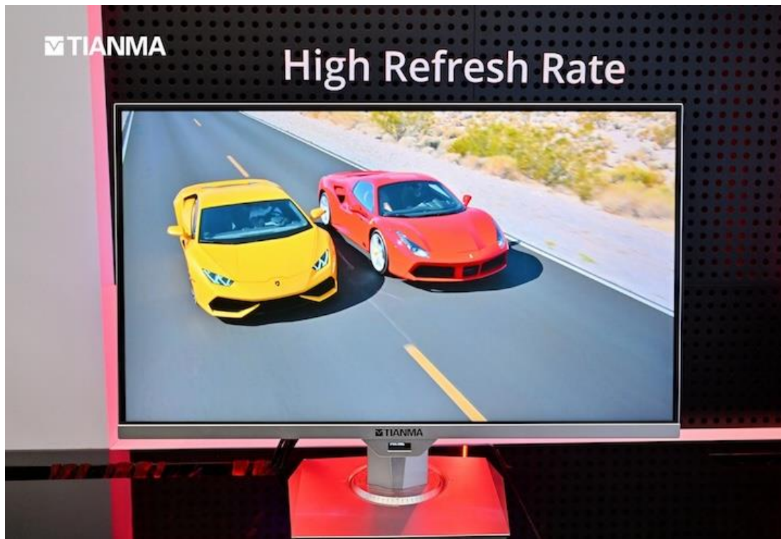
Caption: Tianma 27" QHD 610Hz Oxide Display World's Fastest Native Refresh Rate Oxide LCD Panel
