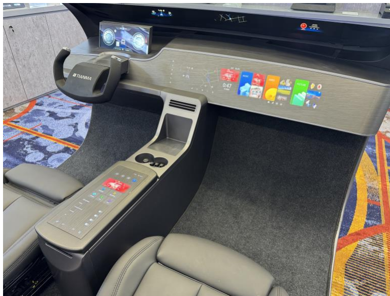
Tianma's Cockpit Demo features: a 12.3" 3D Instrument Cluster; 12.3" LTPS High Transmissivity InvisiVue™ Mini-LED; and Integrated Reflective Imaging System (IRIS) Panoramic-HUD.
